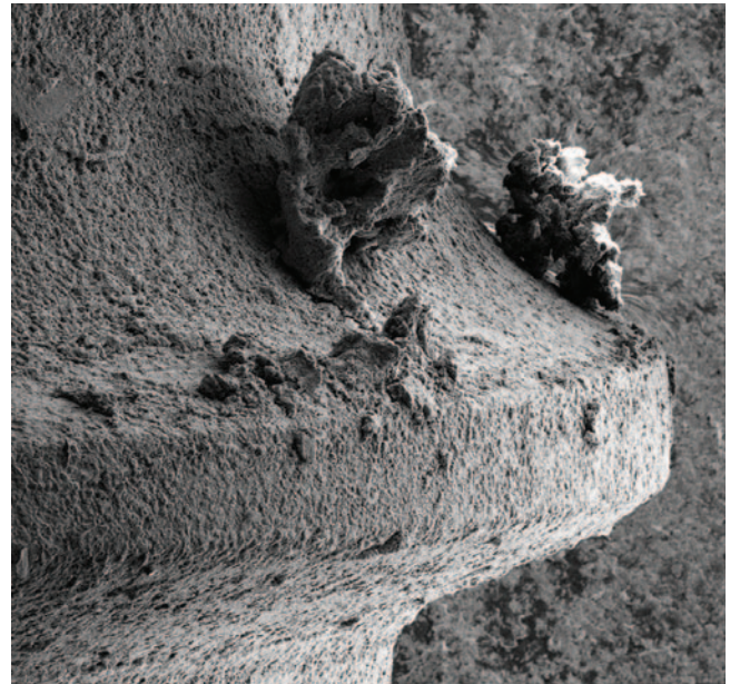
Fig. 1 Bone cells are attached to a titanium surface that was functionalised with a biomimetic to enhance osseointegration. The implant surface is presented after two months in vivo and after removal torque test (TEM picture)
